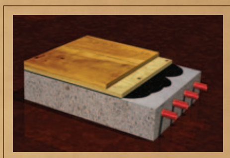
RADIANT HEAT IN CONCRETE SLAB - OPTION 2
