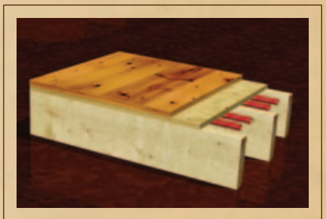
PLYWOOD SUBFLOOR WITH RADIANT UNDERNEATH
